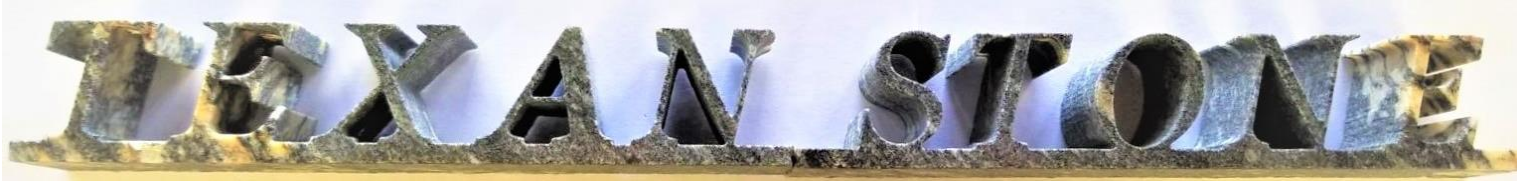
"TEXAN STONE" waterjet cutting with STAR-O-RIGHT
